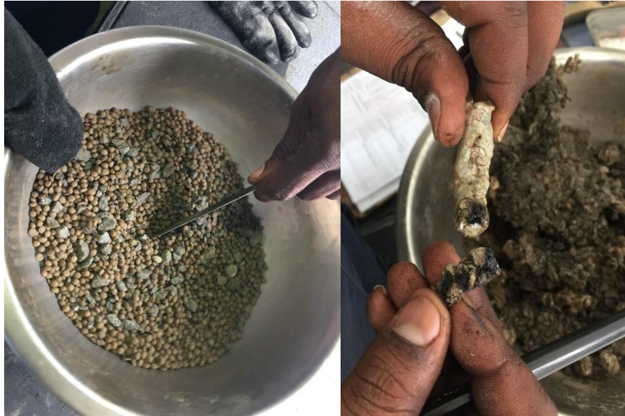
Figure 3: Different forms of waste plastic used in asphalt mixtures (a) Waste plastic pellets: Uniformly sized and (b) Waste plastic crumbs: Irregularly shaped particles
