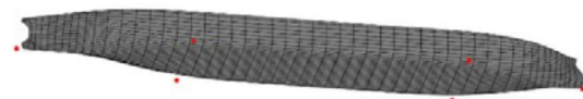
Figure 3 Panel model example of a design vessel and corresponding critical keel point locations in red dots.
