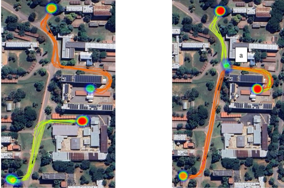
Figure 18. Simulated vehicle interaction heatmap for synthetic routes: (a) separated loading and unloading routes; (b) separate routes leading to a common unloading zone.
