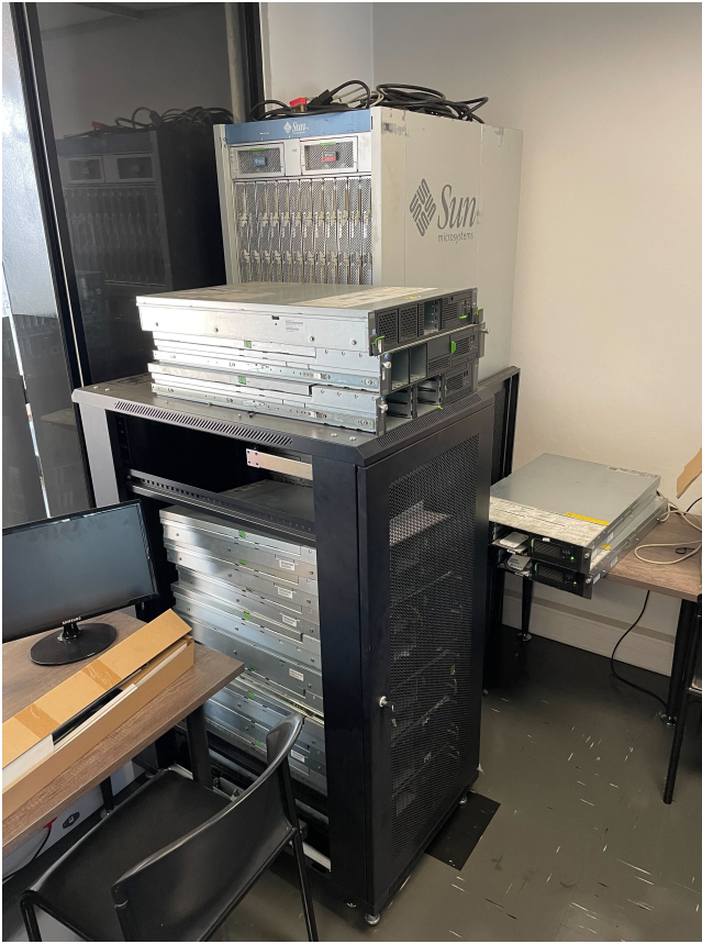
Figure 1: The decommissioned servers we use for training. These servers have DDR3 RAM and Intel XEON E5-2650 Sandy Bridge CPUs.
