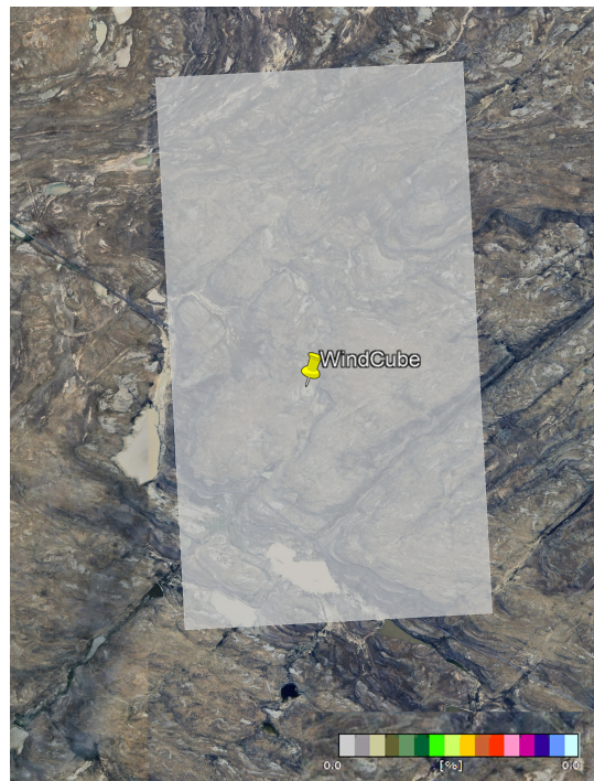
Figure 3 RIX-values in the area surrounding the meteorological mast and LiDAR, confirming that the critical slope is not exceeded.
