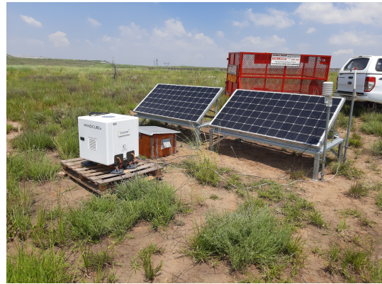
Figure 2 A typical LiDAR deployment site showing the WindCube V2 unit in the foreground with ancillary equipment and the transport vehicle in the background.
