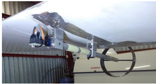
Figure 8. Annular wing exciter mounted on a glider wing
