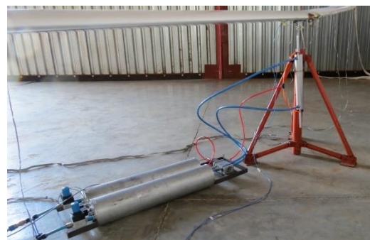
Figure 6. A pneumatic exciter connected to a glider wing, with accumulators in the foreground
