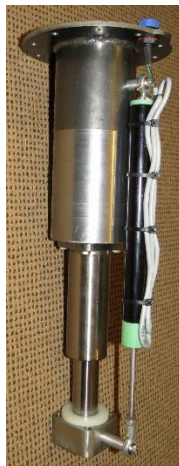
Figure 3. Central column of the vacuum support
