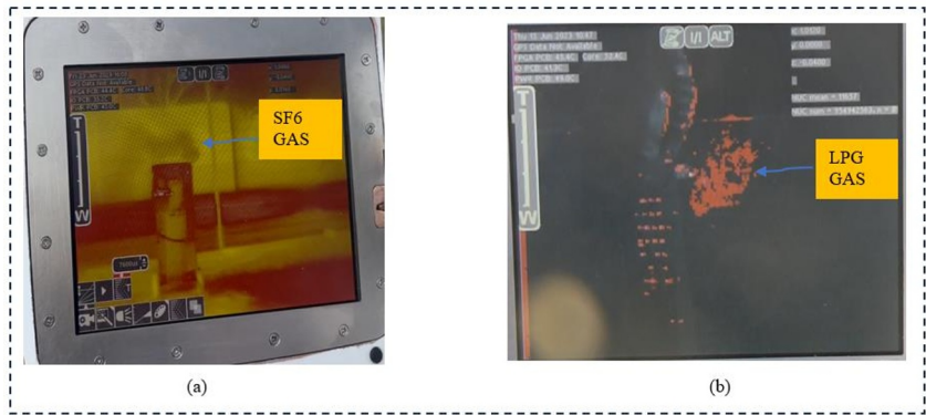
Fig. 9. Optical gas detection (a) SF 6 gas detection (b) VOC - LPG gas detection.
