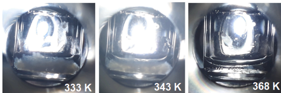
Images taken during the melting progression of Wax 2 at 25 MPa
