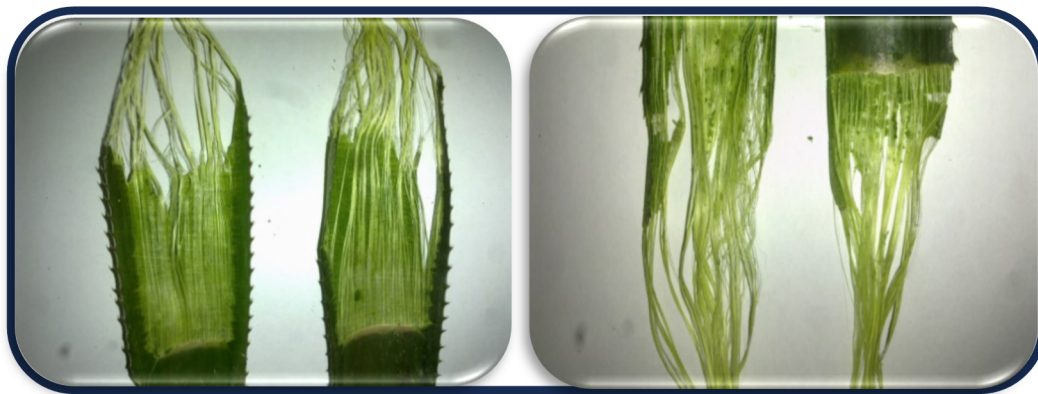
Figure 5. Shows the view of the wet fiber obtained after the extraction process.
