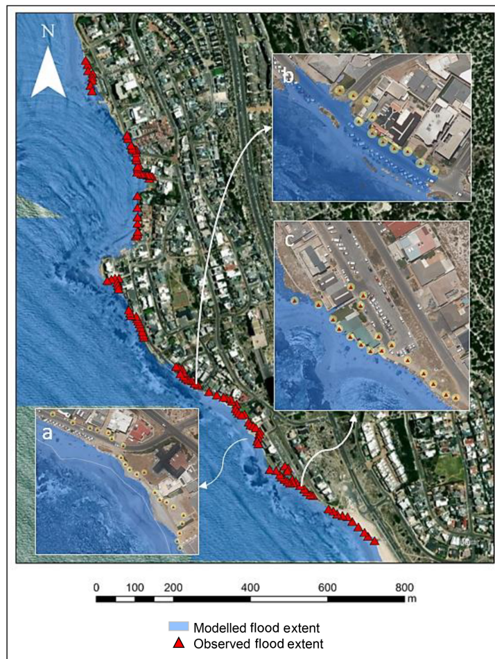
FIGURE 5 | Modeled flood extent and validation points for Bloubergstrand; (a) areas of underestimation; (b) areas of correct model outputs; (c) areas of under- and overestimation.
