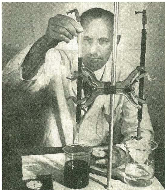
A technologist in the South African Bureau of Standards determining chemical damage to cotton materials by means of a fluidity test.
