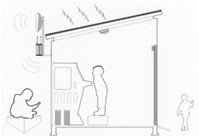
Figure 3: DD housing. Profile drawing depicting solar elements, communication equipment, housing elements and user interactions with the terminals and Wi-Fi access point
