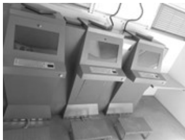
Figure 4 Interior user terminals and management module display embedded in a custom steel housing
