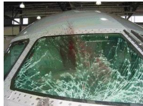
Bird hit damage on aircraft window
