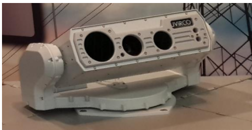
VMI – Vehicle Mounted Inspection system (UV+IR+HD Video + Optical Tracking)
