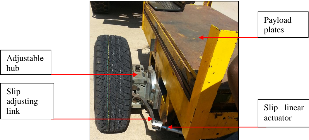
Figure 2: Test setup (with actuators and adjustable hub) for the tyre characterisation of the Dunlop GranTrek AT1 tyre
