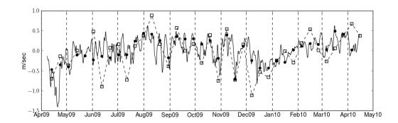
Figure 7: Comparisons between the high resolution along-track altimetry and the ADCP projected velocities at a depth of 30m. The along-track altimetry dataset is plotted with a stippled black line and square markers. The ADCP velocities are plotted in a solid black line, with round markers indicating ADCP observations closest in time to the altimeter's data acquisition. Positive values are indicative of a flow towards the north-east.
