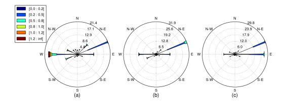
Figure 6: Current rose derived from the ADCP observations for the upper (a), intermediate (b) and lower (c) levels of the water column. Colour bands indicate current speed ranges in  $ms^{-1}$ . Values around the concentric circles show the percentage of time ocean currents are flowing towards a particular direction, with the longest spoke showing the current direction with the greatest frequency.
