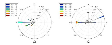
Figure 8: Current roses at the ADCP mooring location dervived from the weekly AVISO merged altimetry (a) and from weekly averages of ADCP observations at a 30m depth (b).
