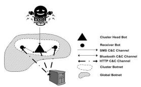
Figure 2: Topology of the Hybrid Mobile Botnet prototype
