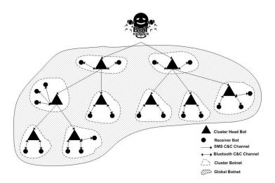
Figure 1: Topology of the Hybrid Mobile Botnet
