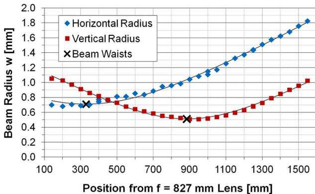
Fig. 5. (Color online) Horizontal and vertical second moment beam radii as functions of distance from an  $f = 827$  mm lens combination at maximum output at 50 Hz. The lines are fits of the beam propagation equation to the measured data and the crosses are the fitted beam waists.
