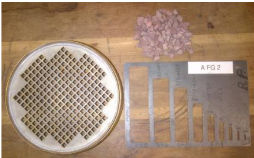
Figure 2.2: Flakiness index test apparatus.
