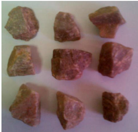
Actual quartzite aggregates
