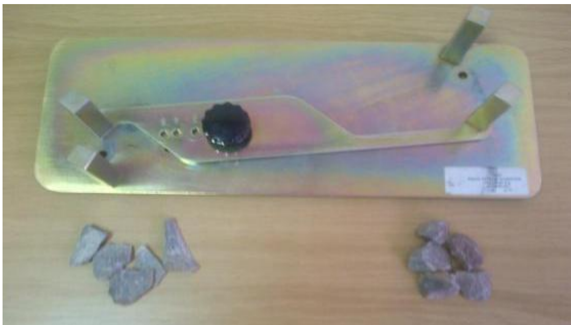
Figure 2.3: Proportional caliper device.
