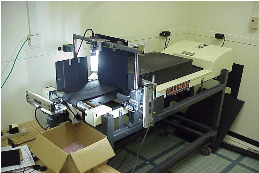
Figure 2.7: The University of Illinois Aggregate Image Analyser (Tutumluer et al, 2003).
