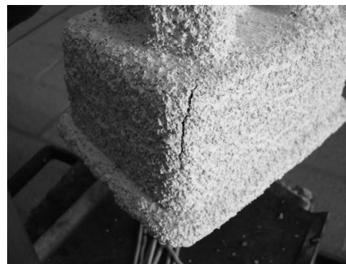
Figure 8: Shell mould after casting showing cracking along the edges.
