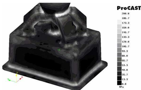
Figure 10: Effective stress profile after casting and simulation using a rigid mould condition.
