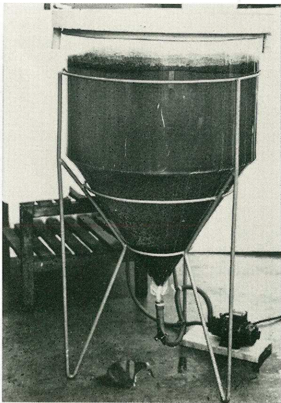
Formation of scum and deposit in effluent from fish factories in an experimental settling tank
