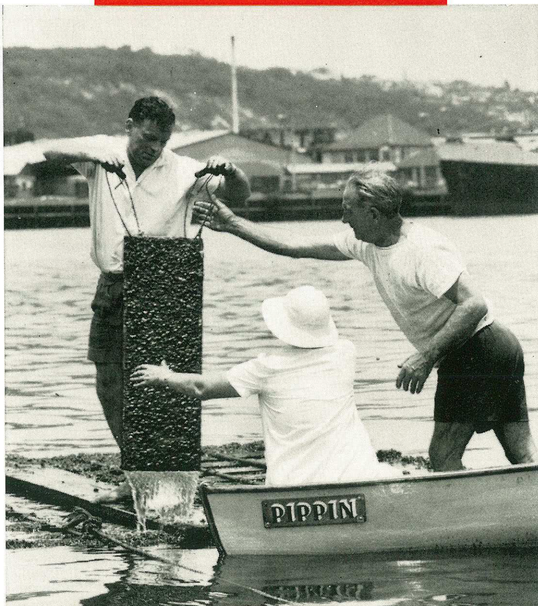
Examination of test panels for anti-fouling paints
