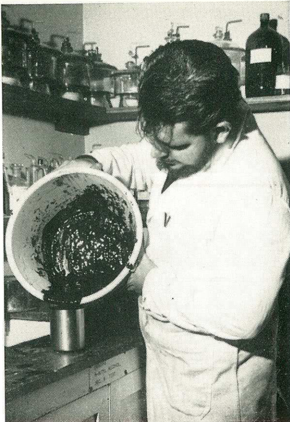
An oil well drilling mud lubricant being prepared for testing after the high pressures and temperatures experienced in deep drilling
