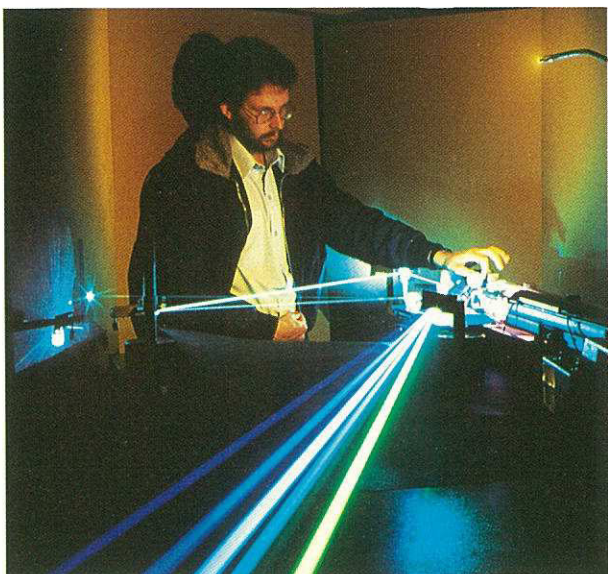
An argon laser at the National Physical Research Laboratory — the laser has become an indispensable tool in certain fields of scientific research.
