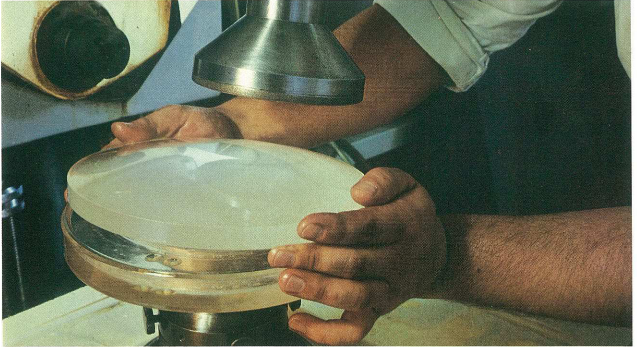
1. Preforming of a lens substrate on a curve generator recently installed at the National Physical Research Laboratory. With a diameter of some 215 mm, this is the largest optical element manufactured to date in South Africa.
