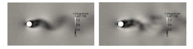
Figure 1. Velocity magnitude contours (shading) and pressure contour (lines spaced at 0.06 Pa intervals between -0.6 Pa and 0.6 Pa), comparing the full finite-volume solution (left) with the adaptive ROM solution (right) at the end of the simulation (75 s).
