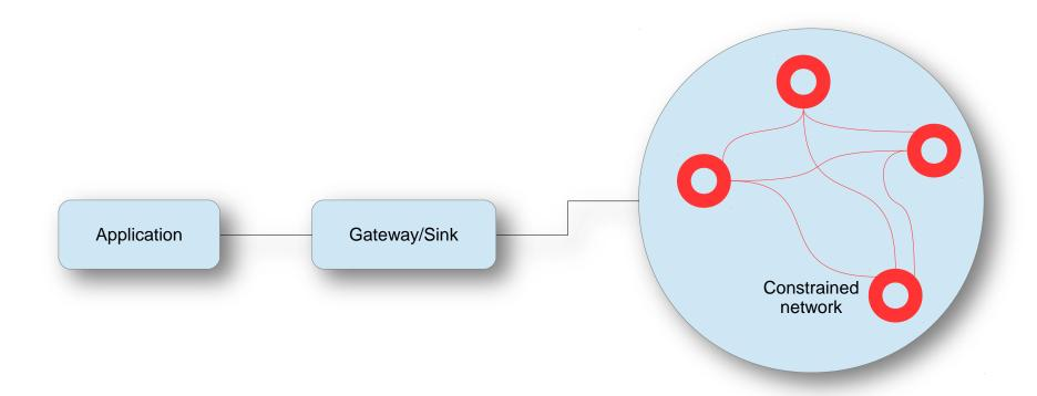
Gateway/Sink node acquires and aggregates data from constrained network and pass it to applications
