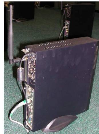
Figure 5. A closer look at an individual node. The RS232 connector is just above and next to the white/green
