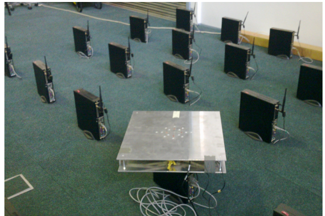
Figure 4. Picture showing the position of the antenna in the node and an overview of the wireless mesh network laboratory
