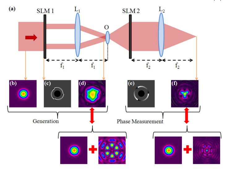
The experiment for extracting the phase delays for each azimuthal mode requires only two SLMs
