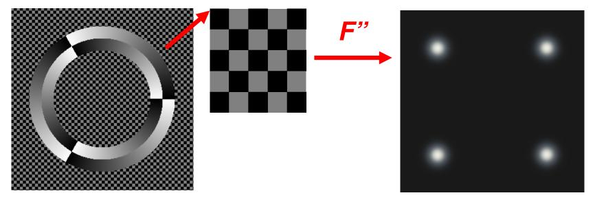
To decompose the azimuthal modes as a function of the radial coordinate, an annular ring restricts the azimuthal match-filter
