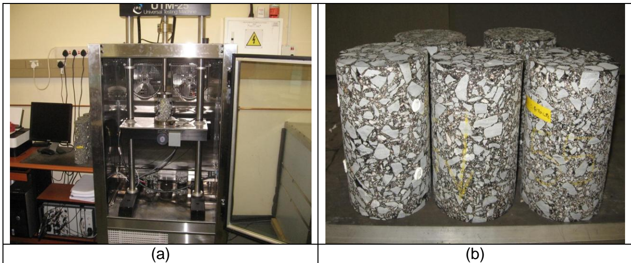
Figure 4: (a) UTM-25 set up at the CSIR, (b) dynamic modulus test samples
