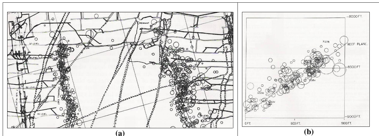
Figure 7. (a) Plan (1000 ft grid) of F longwall East and G longwall West, ERPM, and the foci of 445 seismic events. (b) Dip section of F longwall East, ERPM, and foci of located seismic events. Figures from Cook et al., 1966.
