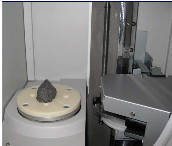
(a) 3D laser scanning device at CSIR BE (b) Sample aggregate on rotating table
