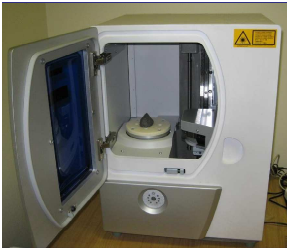
(a) 3D laser scanning device at CSIR BE (b) Sample aggregate on rotating table
