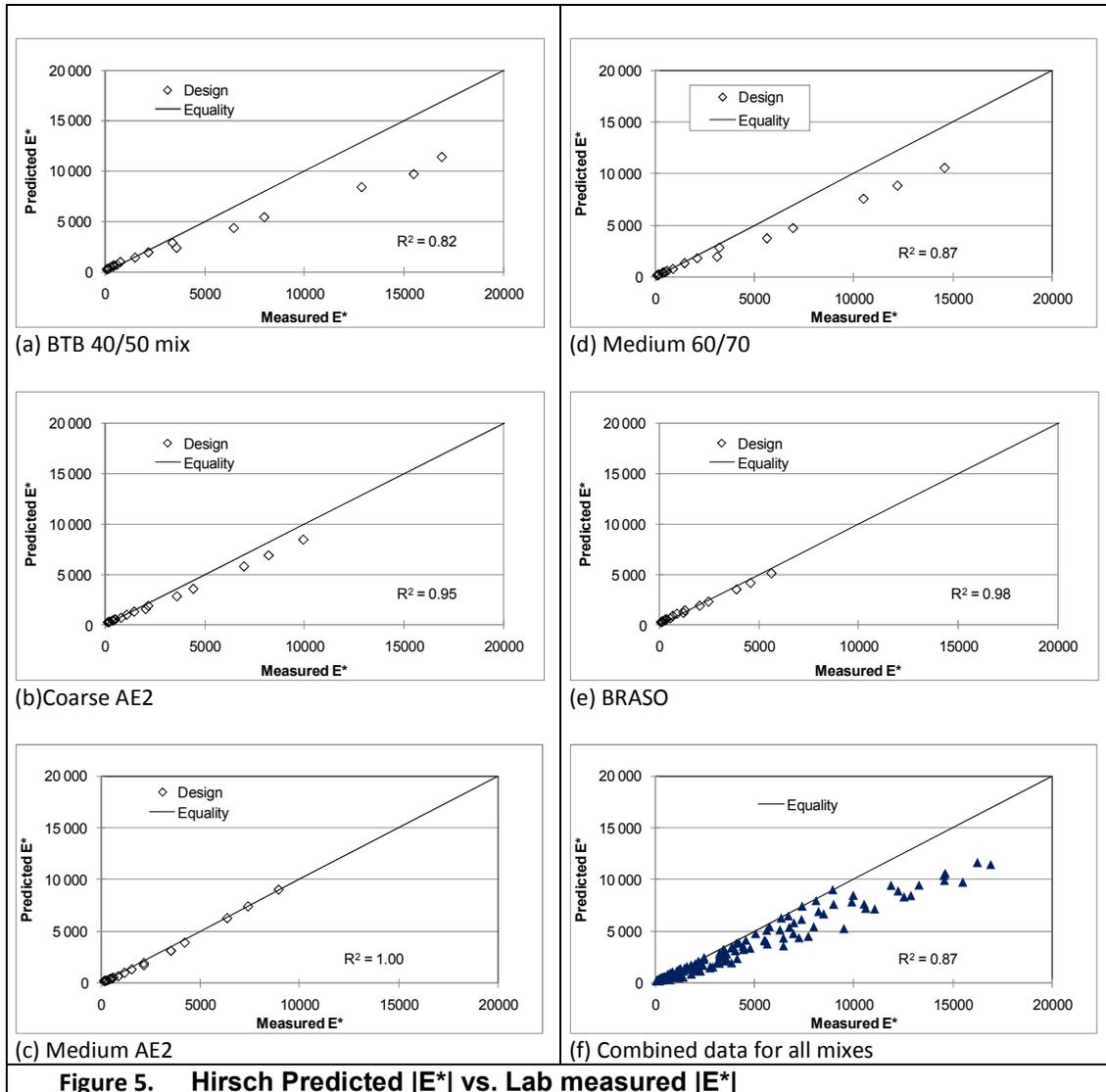
Figure 5. Hirsch Predicted  $|E^*|$  vs. Lab measured  $|E^*|$
