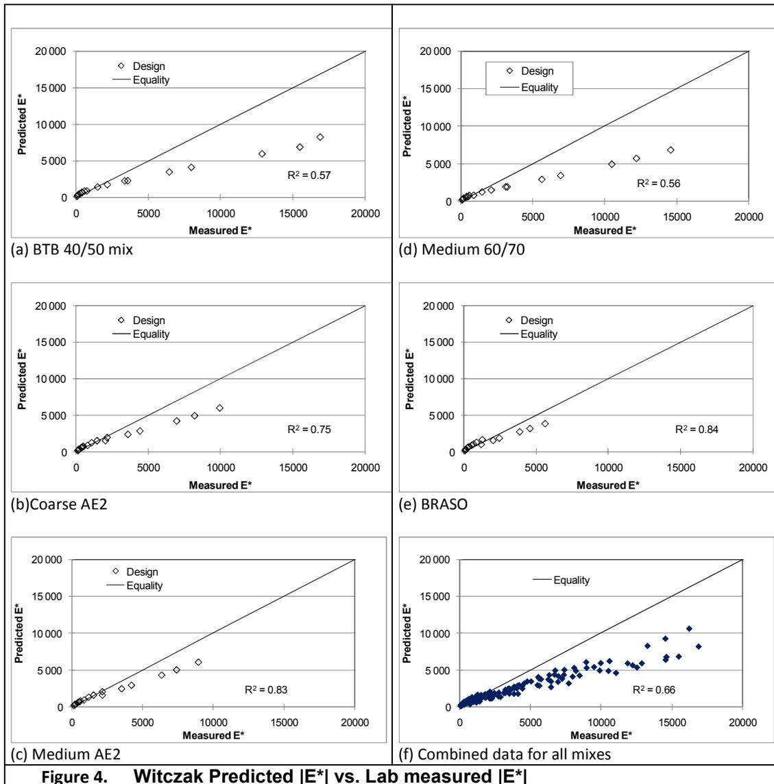
Figure 4. Witczak Predicted  $|E^*|$  vs. Lab measured  $|E^*|$
