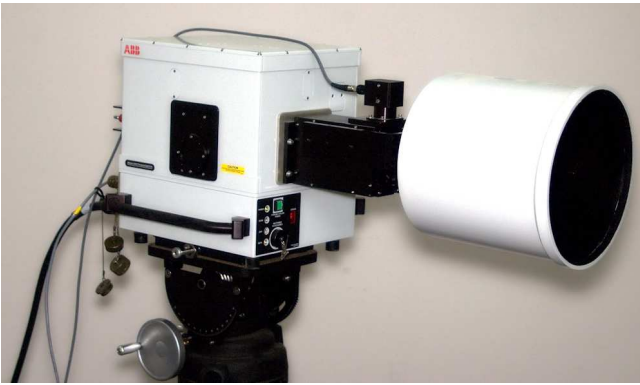
Fig. 3. ABB MR304SC fast scanning mid-infrared spectroradiometer
