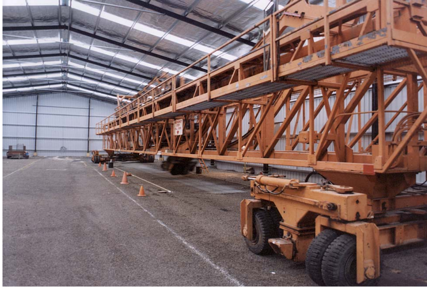
FIGURE 1 ALF operating indoors at a site in Melbourne.
