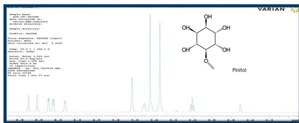
Figure 3.2: 600 MHz <sup>1</sup>H NMR spectrum and structure of pinitol
