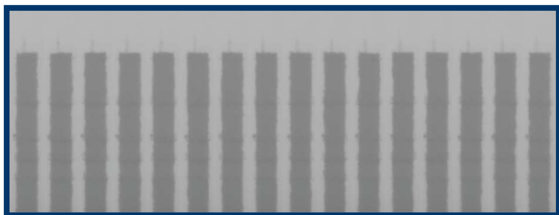
Figure 1: A montage of parts of 16 consecutive video frames captured (40ms apart) by a long range surveillance camera showing the dynamic influence of scintillation on the objects in the images.
