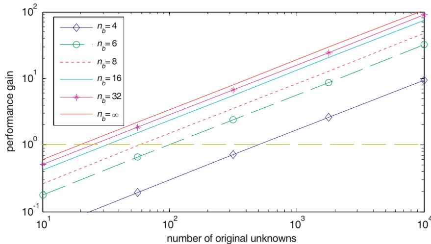
Figure 1. Maximum performance (relative acceleration with respect to the direct MoM) gain versus number of unknowns in the direct MoM;  $n_b$  stands for the number of basis functions assigned per geometrical segment.
