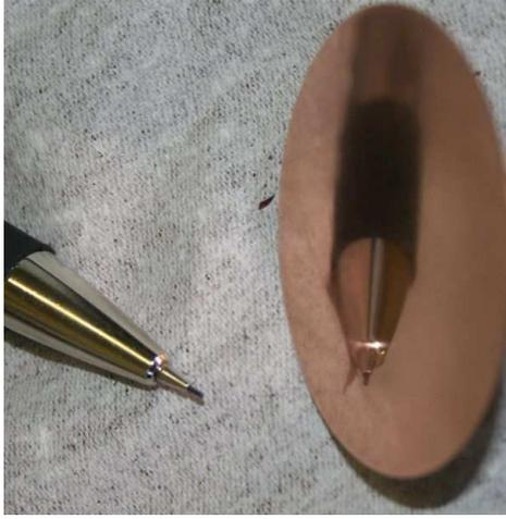
(a) Deformable mirror prototype (front view).
