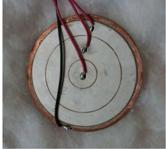
(b) Deformable mirror prototype (rear view).
