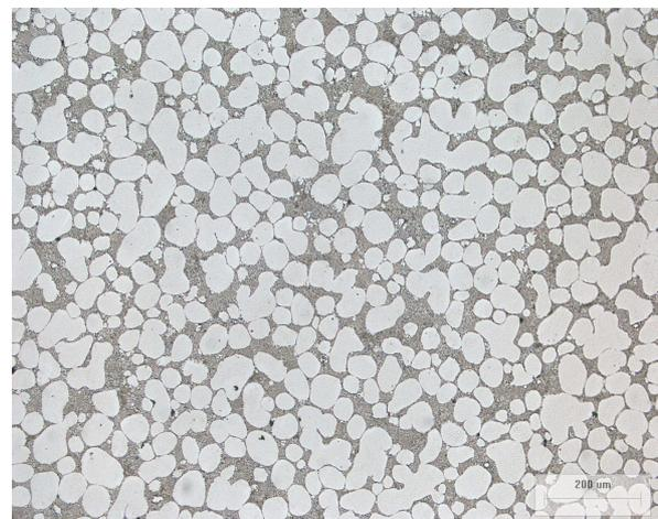
Fig. (2). Typical optical micrograph of SSM HPDC alloy A356 (with 0.31% Mg)
