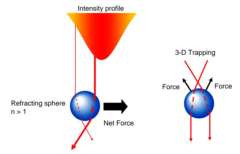
High numerical aperture produces a more tightly focused beam
