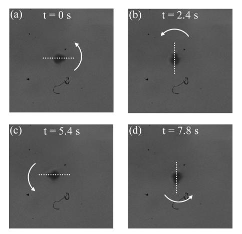
$\omega = 2.77 \pm 0.09 \text{ rad/s}$  $\tau = 1.2 \times 10^{-20} \pm 0.2 \times 10^{-20} \text{ Nm}$  Technique can be used in microfluidics to precisely measure fluid parameters
