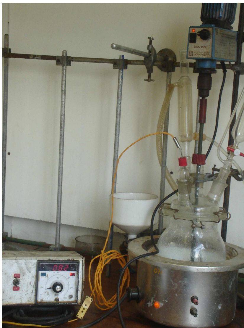
Figure 4.1: The experimental set up for the sol-gel preparation
