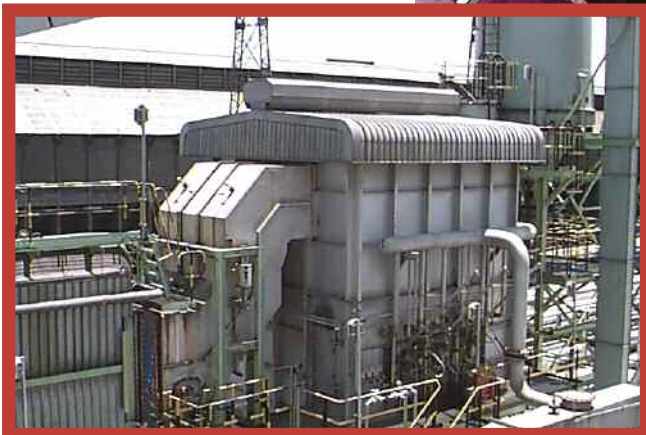
The high sulphur pitch incinerator built for a South African petrochemical company
