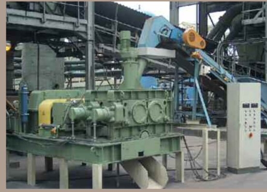
Briquetting Press: The machine used to produce briquettes
