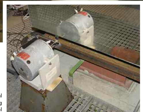
Mechanical vibration testing of mirror panel
