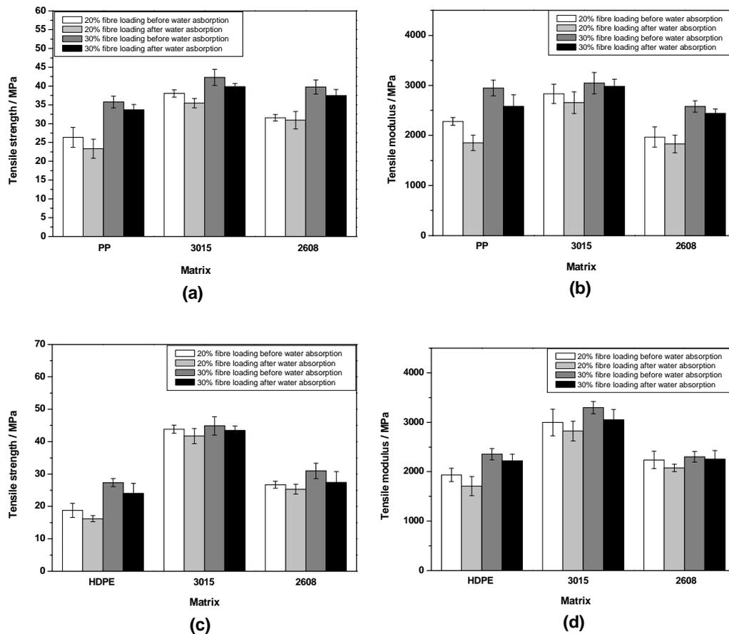
Figure 3. The variation of tensile properties of hemp/PP and HDPE composites, before and after water immersion with two different types of compatibilizers. (a) and (b) tensile strength and modulus of PP/hemp fibre composites; (c) and (d) flexural strength and modulus of the HDPE/hemp fibre composites .
