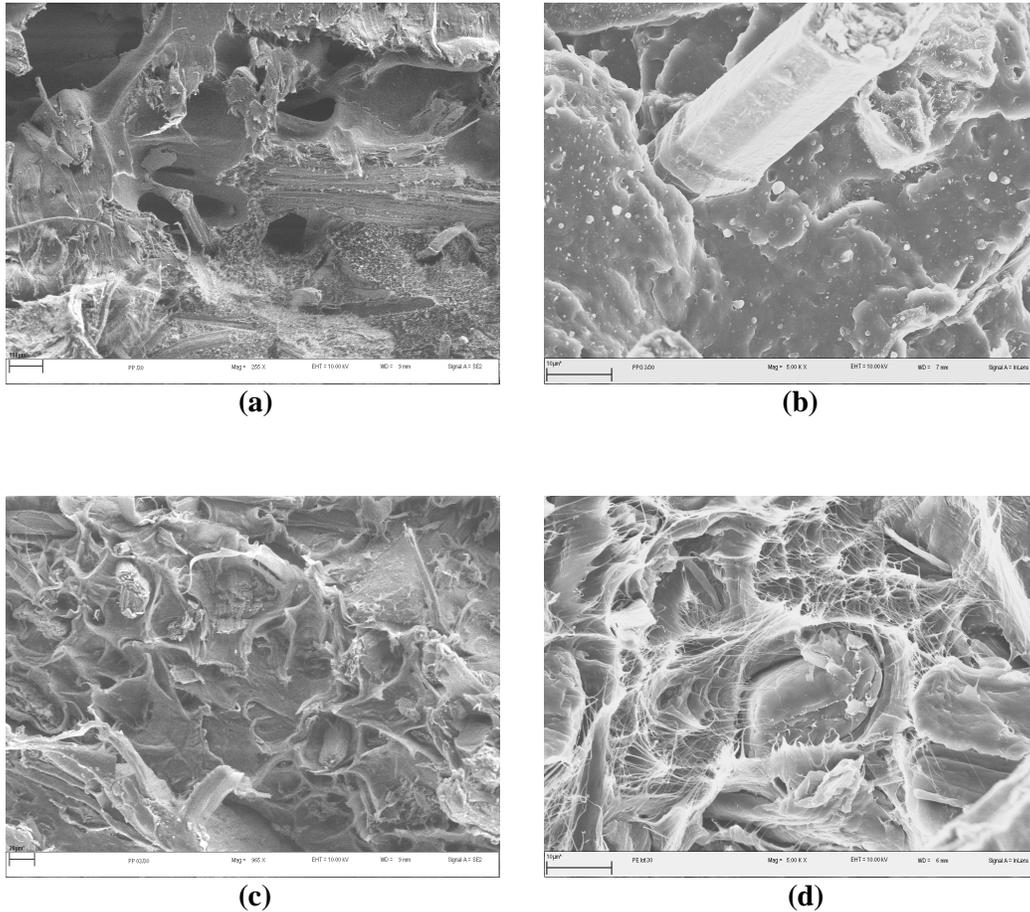
Figure 6. The SEM micrographs of hemp fibre composites, (a) and (b) 30% hemp fibre/PP composites and (c) and (d) 30% hemp fibre/PP composites with compatibilizer
