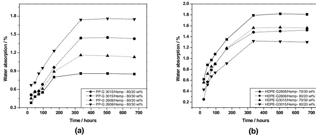
Figure.2. The variation of water absorption on PP and HDPE/hemp fibre composites with different compatibilizers, (a) PP/hemp fibre composites and (b) HDPE/hemp fibre composites
