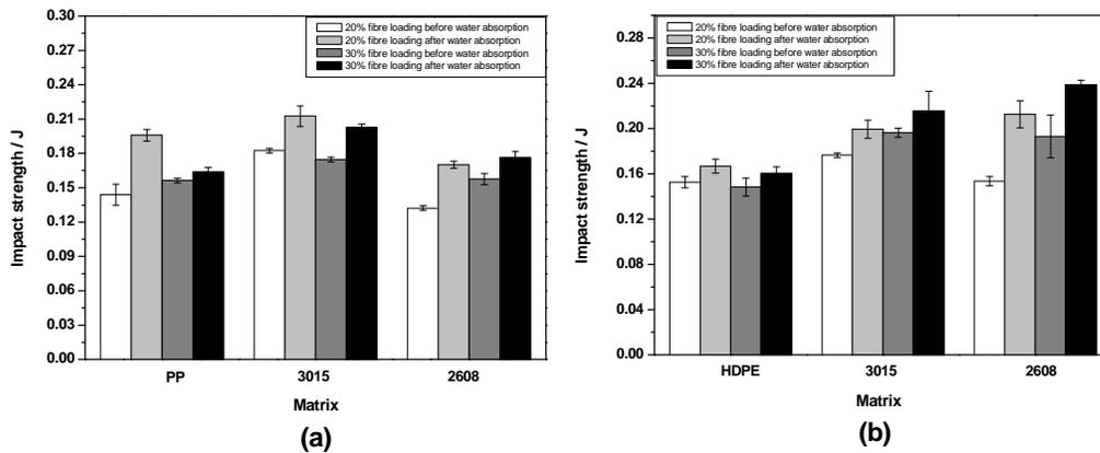
Figure 5. The variation of impact strength of the composites before and after water immersion with two different types of compatibilizers (a) PP/hemp composites with PP-g-MA and PE-g-MA and (b) HDPE/hemp composites with PP-g-MA and PE-g-MA.
