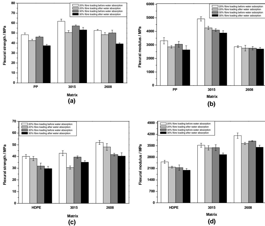
Figure 4. The variation of flexural properties of hemp/PP and HDPE composites, before and after water immersion with two different types of compatibilizers. (a) and (b) tensile strength and modulus of PP/hemp fibre composites; (c) and (d) flexural strength and modulus of the HDPE/hemp fibre composites
