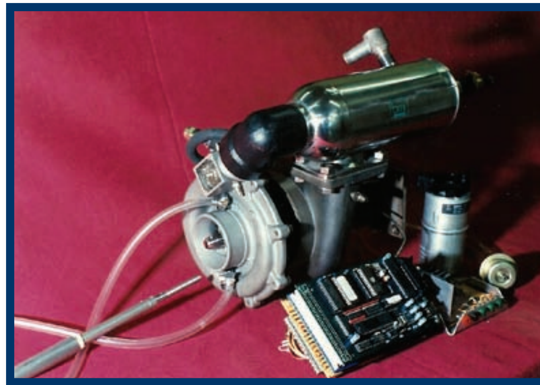
Figure 3: Core of microturbine technology demonstrator
