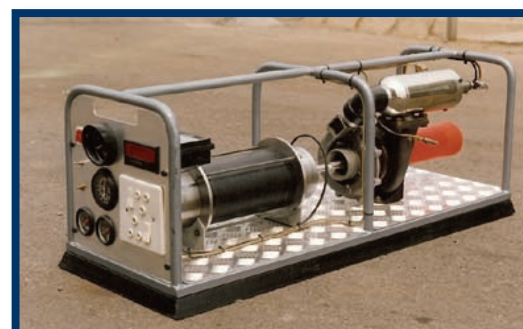
Figure 4: Mock-up of directly coupled microturbine/alternator
