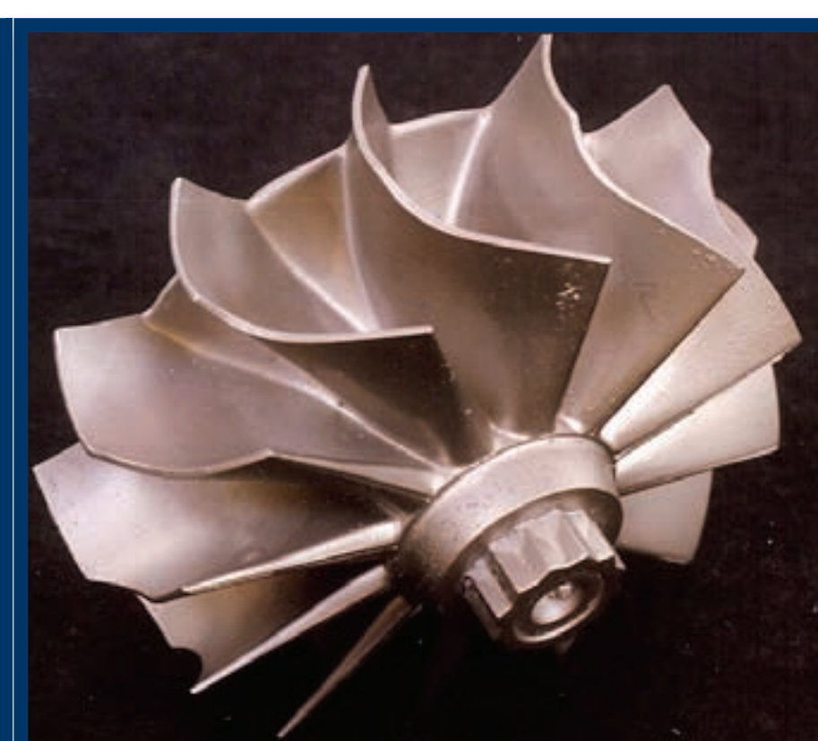
Figure 6: Superalloy casting of radial turbine
