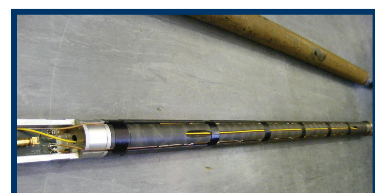
Figure 7: Directional BHR receiver with the four dipole antenna elements in a receiver probe
