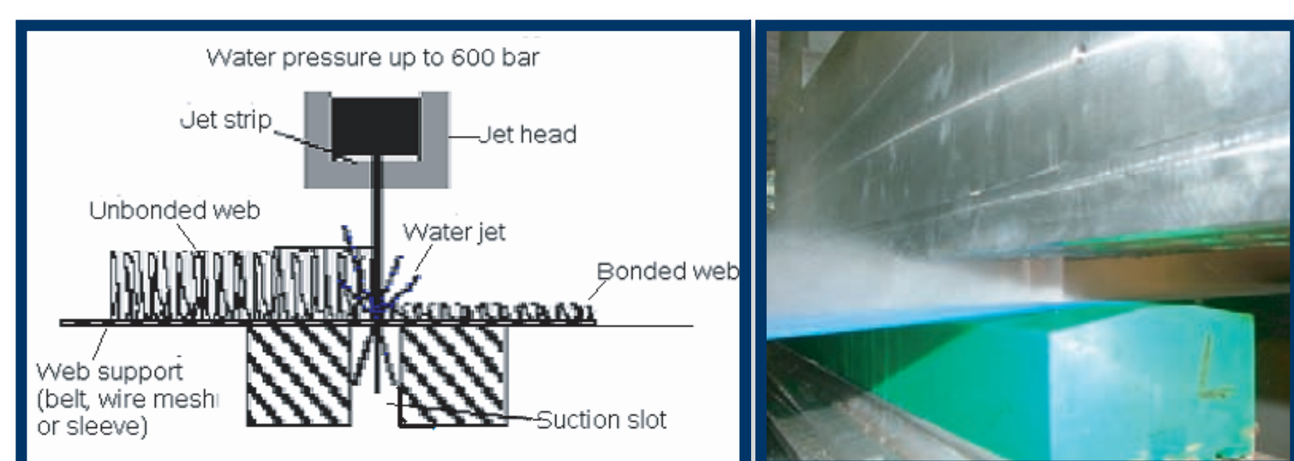
Figure 1. Hydroentanglement process Figure 2. Water jets through a manifold
