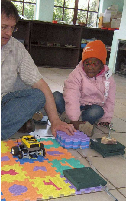
Figure 8: Controlling a toy car using RockBlocks. Here the testee has placed one rock on a programming square (right) to control the toy car (left).
