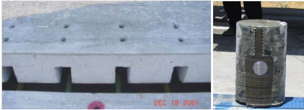
Figure 1. Doweled joint and core showing dovetail slot/dowel bar connection
