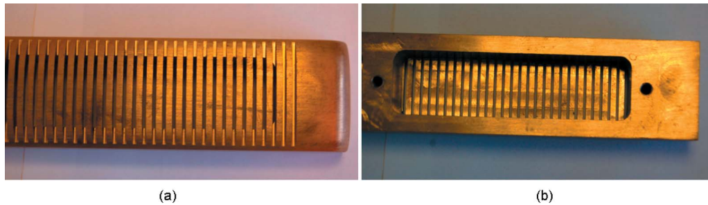
Fig. 7 Slotted discharge electrode as viewed from (a) top and (b) bottom. The electrode employs slots of 1.5-mm width cut at a pitch of 4 mm and is hollowed to allow for a suitable damping material to be inserted.
