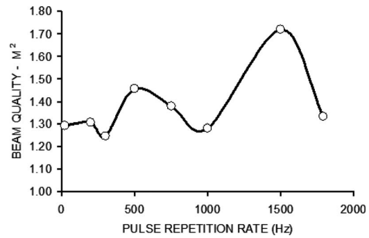
Fig. 10 Laser beam quality factor M^2 of the laser resonator versus pulse repetition rate.
