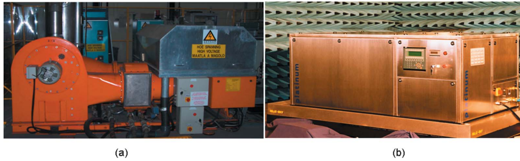
Fig. 1 (a) The 2000-Hz system, showing the blower system to the left and the laser head to the right. (b) The commercial 400-Hz system designed specifically for laser ultrasonic testing of materials.
