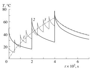
**Fig. 1.** Heating kinetics at points located on the axis of a laser beam on the outer boundary of a blood layer for (2) three and (3) nine pulses per series. Curve 1 shows the same dependence for a rectangular pulse with a duration of 0.04 s.
