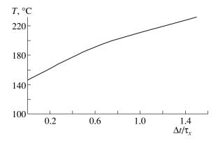
**Fig. 4.** Maximal temperature (°C) of the outer surface of an absorbing layer corresponding to the threshold coagulation conditions on the inner surface as a function of the pulse repetition period in the series. The calculation performed taking into account the temperature of the medium (36.7°C).
