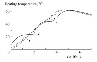
**Fig. 2.** Heating kinetics at points located on the axis of a laser beam on the inner boundary of a blood layer for (2) three and (3) nine pulses per series. Curve 1 shows the same dependence for a rectangular pulse with a duration of 0.04 s.
