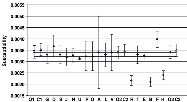
**Figure 2.** Magnetic susceptibility for 1 OIML. Uncertainty bars and median limits, indicated by horizontal lines,  $k = 2$ . Data C1, C2 and C3 represent control standard measurements.
