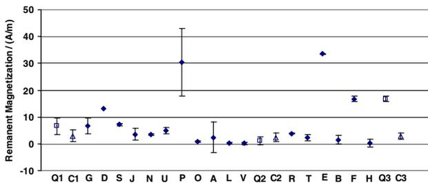
**Figure 8.** Remanent magnetization for [52]. Uncertainty bars  $k = 2$ . Data C1, C2 and C3 represent control standard measurements.
