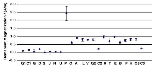
**Figure 3.** The remanent magnetization for 1 OIML. Uncertainty bars  $k = 2$ . Data C1, C2 and C3 represent control standard measurements.
