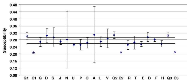
**Figure 4.** Magnetic susceptibility for C&CA. Uncertainty bars and median limits, indicated by horizontal lines,  $k = 2$ . Data C1, C2 and C3 represent control standard measurements.
