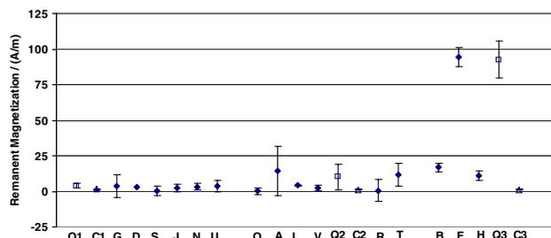
**Figure 6.** Remanent magnetization for C&CA with the ordinate scaled to emphasize dispersion for smaller data; two data are lost as a result. Uncertainty bars  $k = 2$ . Data C1, C2 and C3 represent control standard measurements.
