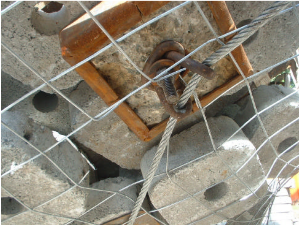
Figure A-39 Initiation of mesh failure in the test on 17/01/02
