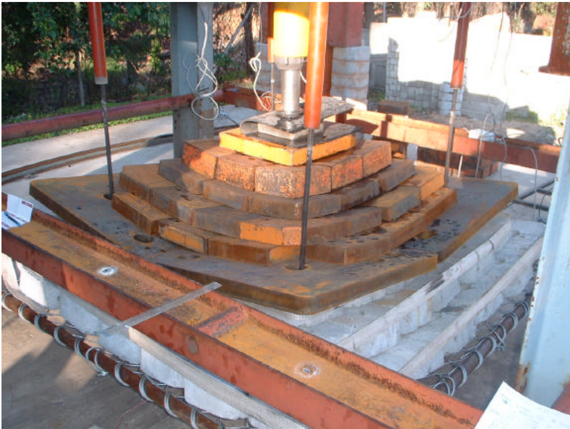
Figure A-2 Yielding of cone bolts at the end of the test on 30/10/01 (indicated by white tape relative to the bottom of the tube)
