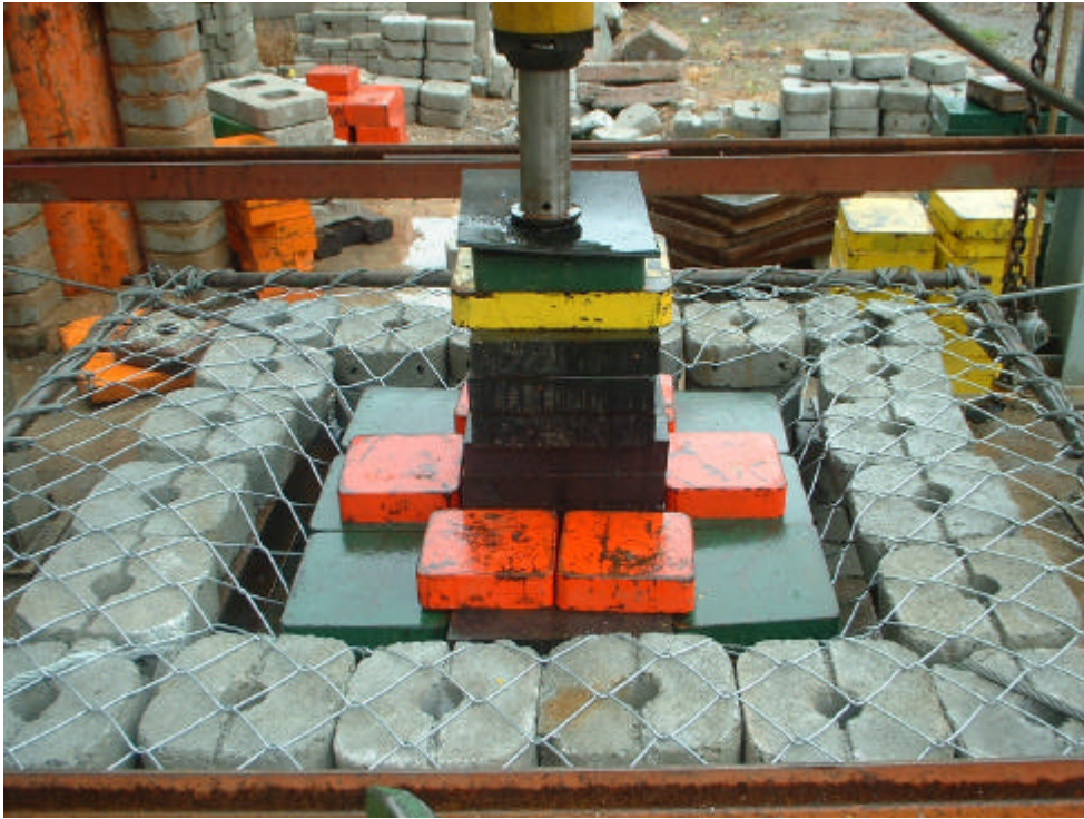
Figure A-27 Failure of mesh and lacing in the test on 14/02/02
