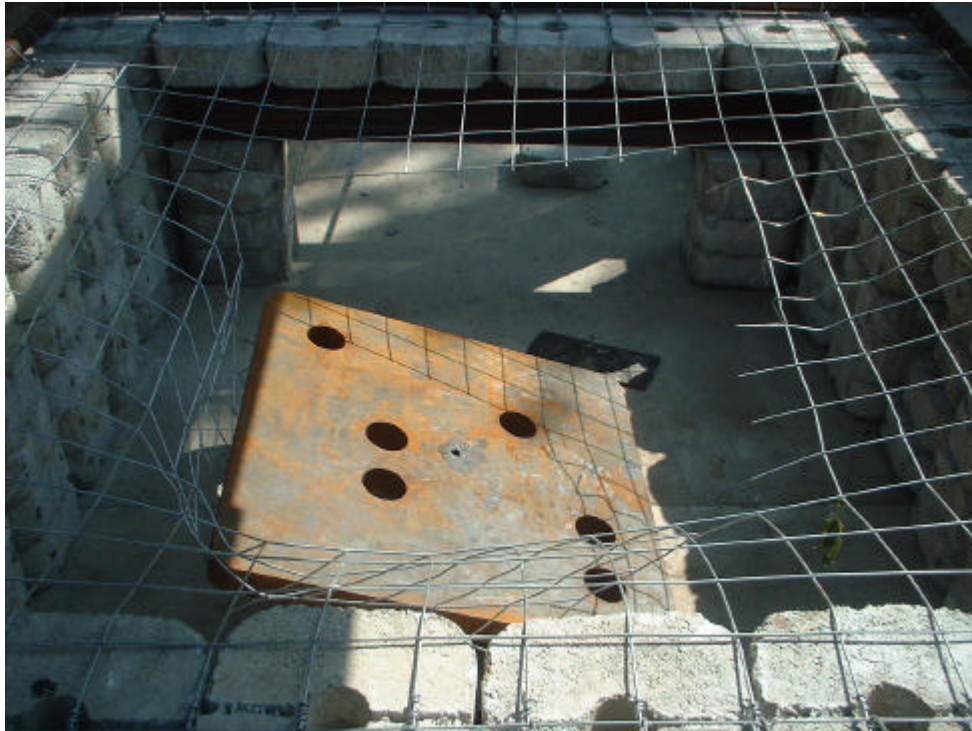
Figure A-33 Mesh failure in the test on 05/03/02
