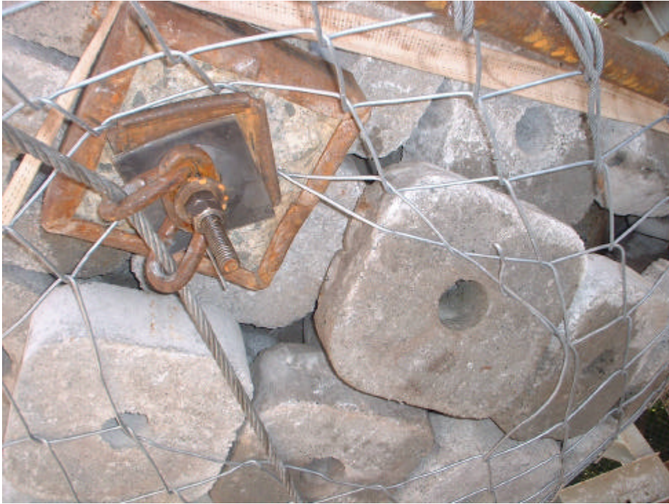
Figure A-59 Mesh failure around bearing plates in the test on 04/03/02
