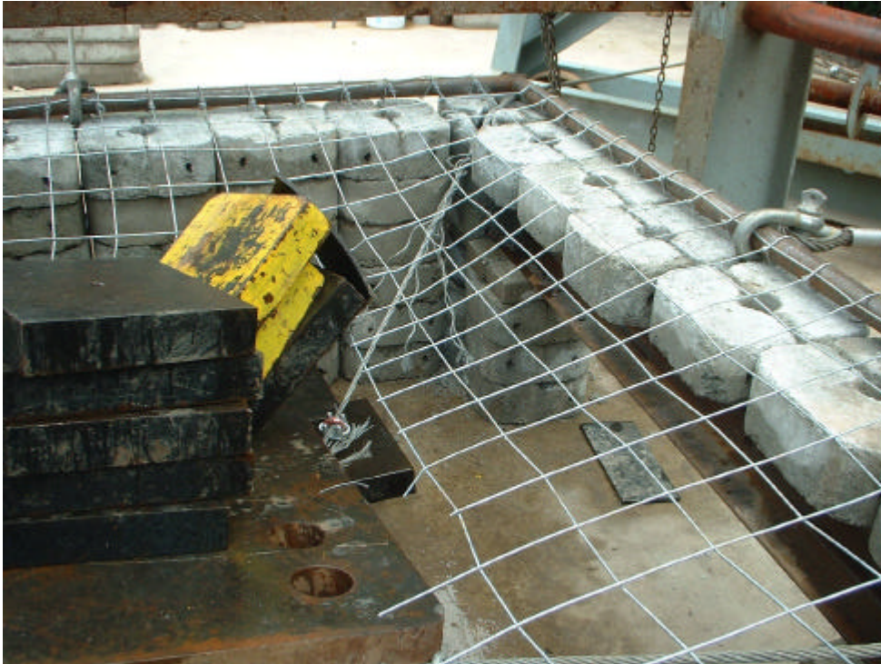
Figure A-34 Mesh and cable failure in the test on 07/03/02
