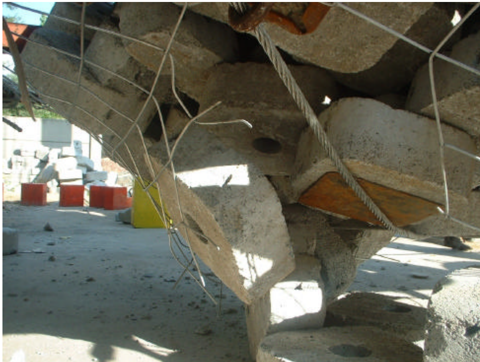
Figure A-38 Mesh failure in the test on 17/01/02
