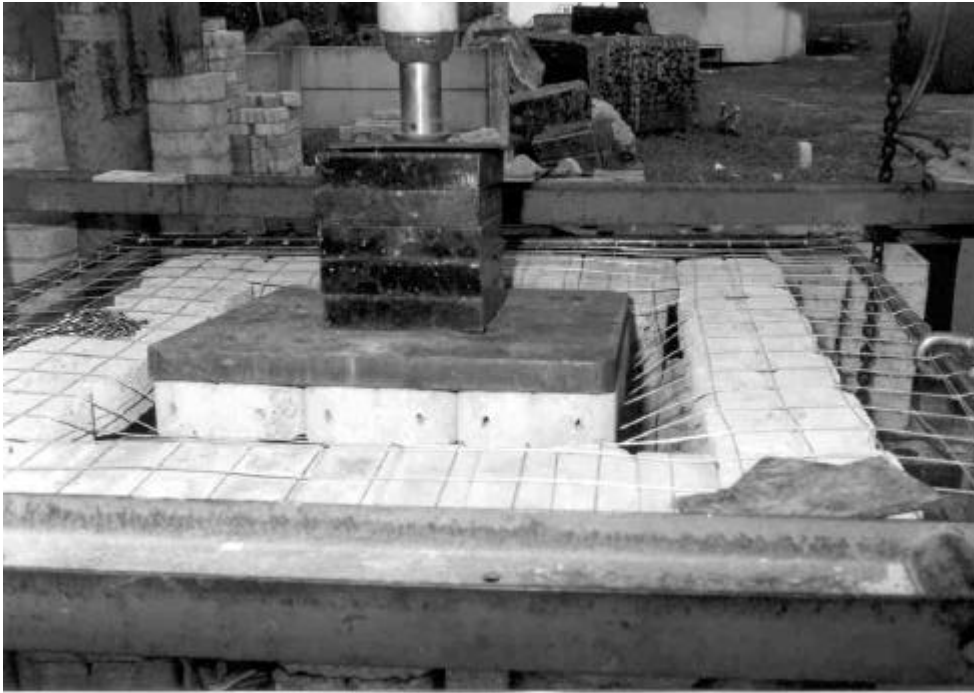
Figure A-23 Failure of welded mesh in test 24/01/02
