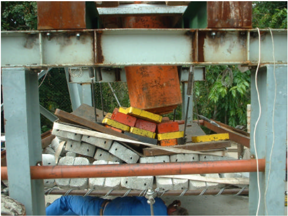
Figure A-60 Rupture of two tendons in the test on 11/03/01
